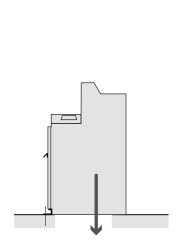
N.B.: parts for guiding the gases to vent openings and cooling walls are not part of the switchgear supply. These must be adapted to each specific case.
