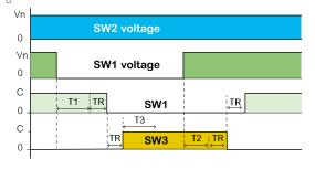
Source changeover between 2 incoming lines (SW1 and SW2) and a busbar coupling switch (SW3)
