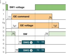
Case (1): Generator channel closing after Generator power on (configurable option)
